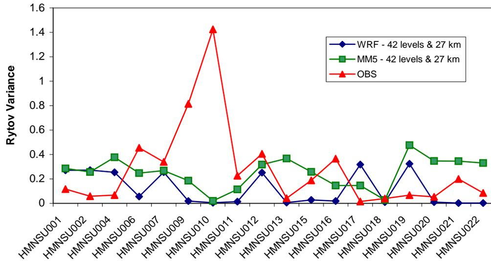
**Figure 1. Rytov variance computed from observed and WRF and MM5 derived  $C_n^2$  profiles for sample laser path for each of the balloon flights in the Holloman Summer 2002 Experiment.**
